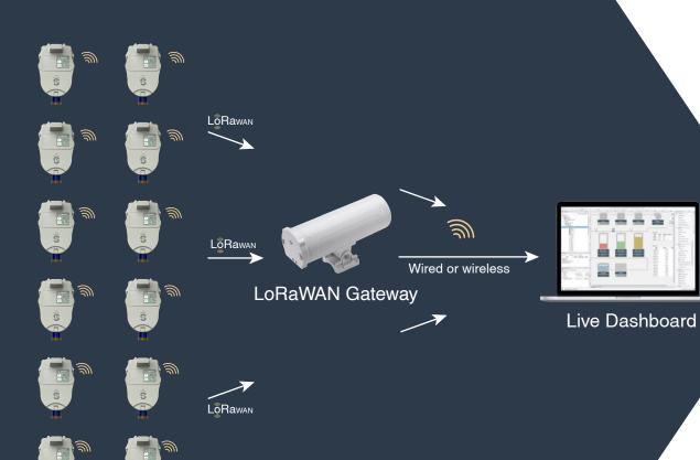
Removing the need for physical meter reading and opportunity for human error with use of NB-IoT or LoRaWAN.
